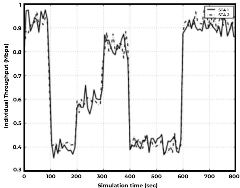
The left figure, on the other hand, shows another key characteristic that contains only two individual throughputs for fixed and varying stations. We can infer that stations observe the same individual throughput. Hence, stations with higher data rate observe the same throughput with the slow station.
