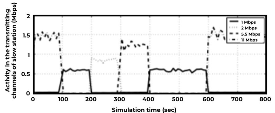
The plot from the above figure shows the activity of the station that changes its data rate. The station starts with 11Mbps data rate, and at  $t=100\text{sec}$ , drops down the rate to 1Mbps until  $t=200\text{sec}$ . Between 200sec and 300sec, the station operates at 2Mbps and for the next 100sec it operates at 5.5 Mbps.
