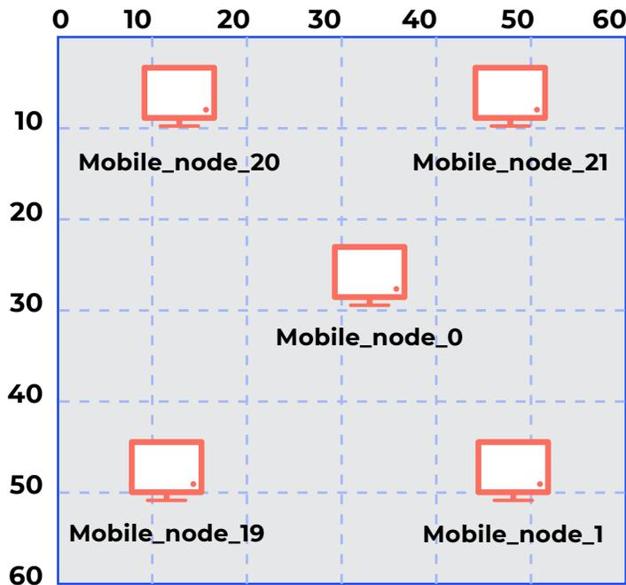
Here we show a simulation in OPNET with a network of five nodes, all with 11 Mbps data rate, but one of them changes its rate with time as a control node.
